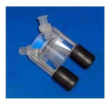
QCMagicHat can be equipped with our plexiglass Liquid Cell, featuring both static and flow-through operations, designed for HC6/U crystals, namely for quartzes featuring blank diameter of about 0.550" and electrode diameter of about 0.295". It is composed by two parts:
