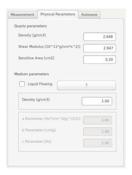
By default, each parameter has values related to an AT-cut quartz crystal. If the instrument is used with liquids, the user must input the medium's density. If the liquid medium flows, the user must input also the a,b, and c parameters, as described above.
