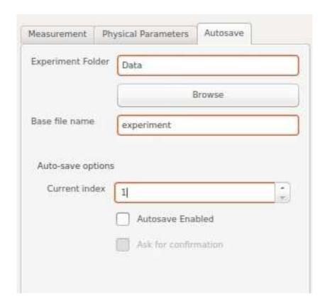
The user, in addition to manually save each single acquisition plot, can automatically save all the acquisition sessions simply indicating the working folder, a base file name and the initial count number. The program will take care of incrementing and adding a numerical suffix when saving data.
