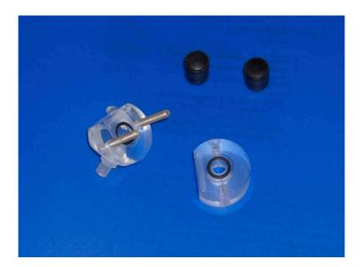
The base part has the quartz fitting place and two (in-out) flow connectors. The top part shows a conical hole for static liquid measurements.
