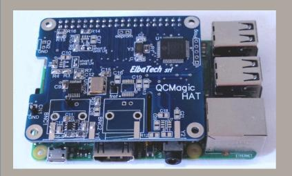
The first plug-n-go module for RaspberryPi featuring a high precision dual-channel Quartz Crystal Microbalance.
